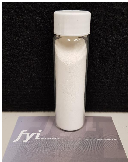
FYI's HPA produced from Cadoux kaolin feedstock (99.997% Al 2 O 3 )
