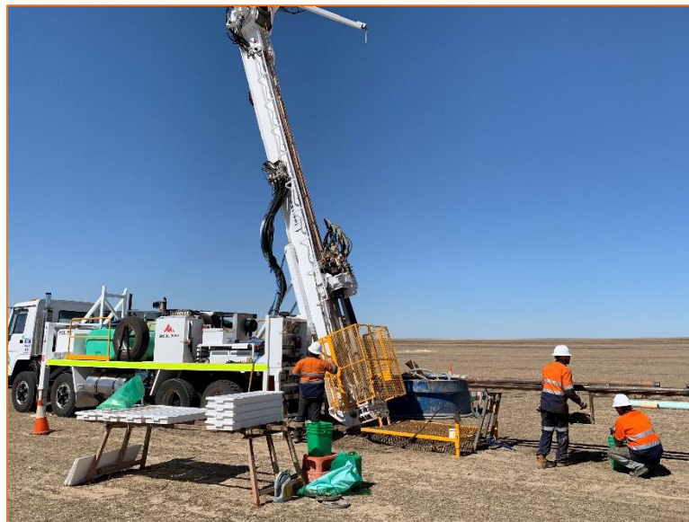
Diamond Drilling at Cadoux HPA Project
