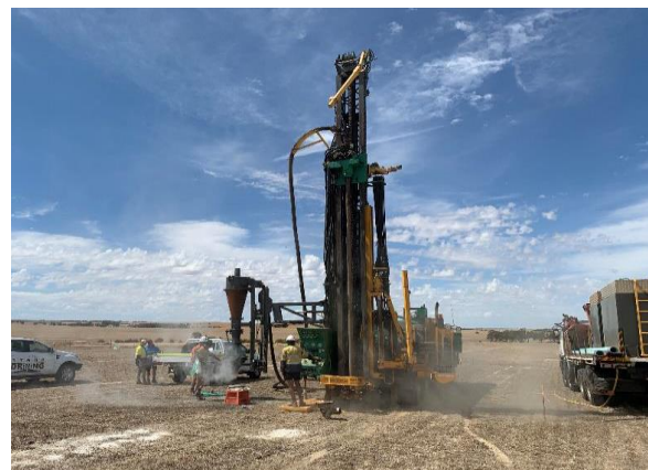
RC Drilling at Cadoux Project
