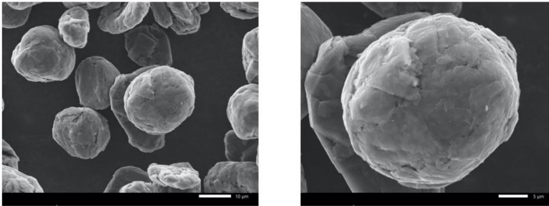
**Scanning electron microscopy of high purity alumina doped coated spherical graphite**
